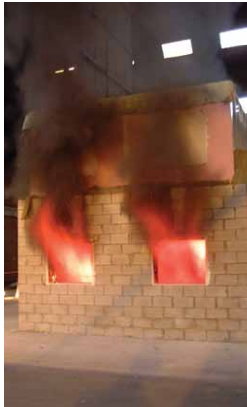
Figure 24 Fire test on light steel frame building
